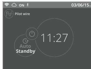
Pilot wire = Stop (Heating standby mode)
